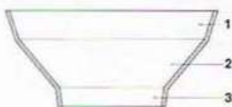
Adaptation of the air-funnel shape. 1 For maximum power, 2 For part load, 3 For idle.
