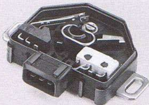
36) Throttle-valve switch for end-position signal.
